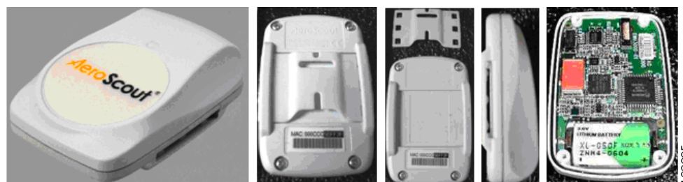
Figure 72 AeroScout T2 802.11 Wi-Fi Active RFID Tag
