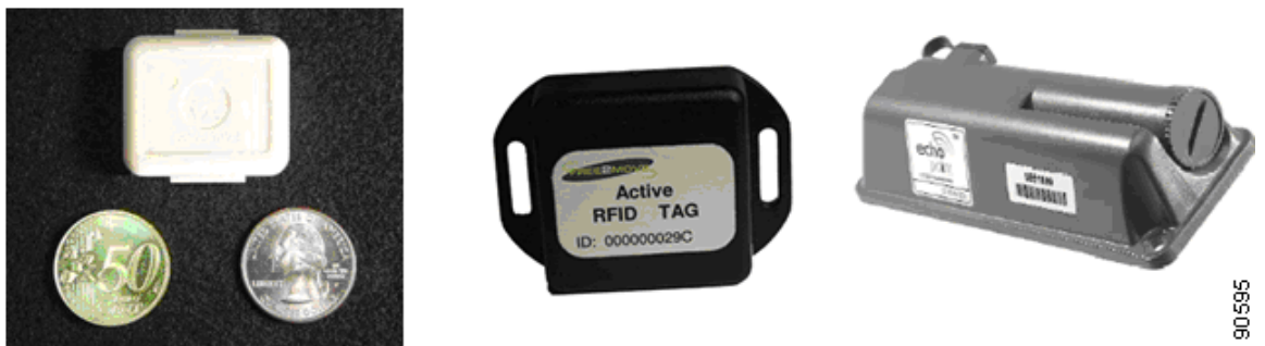
Figure 62 Active RFID Tags
