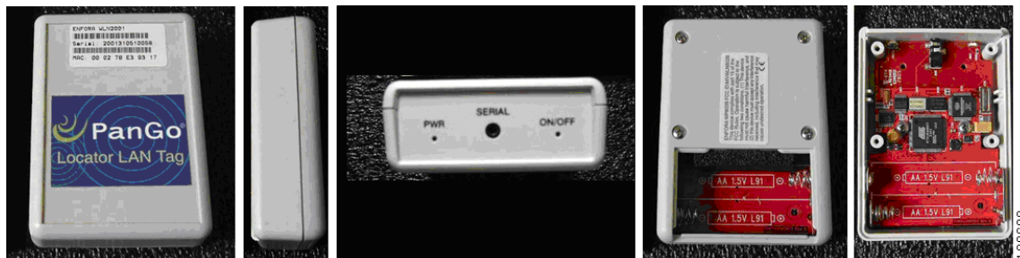
Figure 75 PanGo Locator LAN Tag (Version 1)
